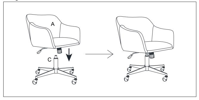
Position the Seat (A) facing down over the top of Gas Lift (C). Insert the Gas Lift (C) into the center hole of Lift Mechanism (B) and press down until fully engaged.
