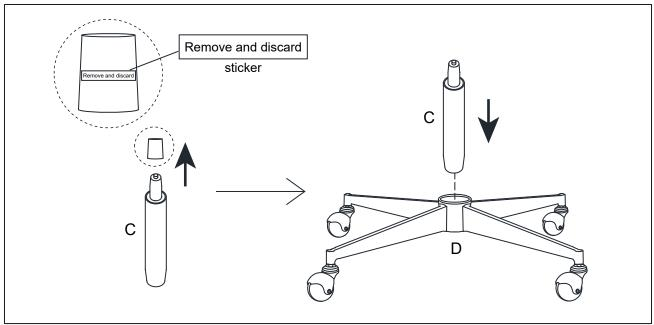
Turn base assembly from previous step right side up, onto casters. Remove and discard plastic cap from Gas Lift (C). Insert Gas Lift (C) into the venter hole of base (D) as shown.
