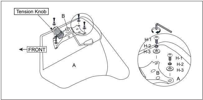
Align holes on Lift Mechanism (B) to pre-threaded holes on Seat (A). Attach Lift Mechanism (B) using Allen Bolts (H-1), Spring Washers (H-2) and Flat Washers (H-3), stacking hardware in the order as shown. Make sure the Tension Knob faces towards the front of chair assembly. Engage Allen Bolts (H-1) using Allen Key (T-1) but do not fully tighten them until insert all 4 bolts to holes.
